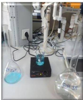
Figure 4. Step 2: Example of solution preparation at pH 3.5
