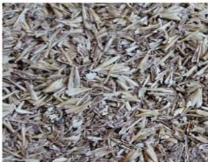
Figure 2: A photo of the brewer's spent grains as a solid waste of beer production
