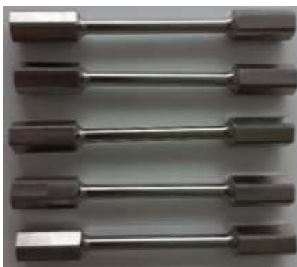
Figure 2. Torsion test specimens machined with turning
