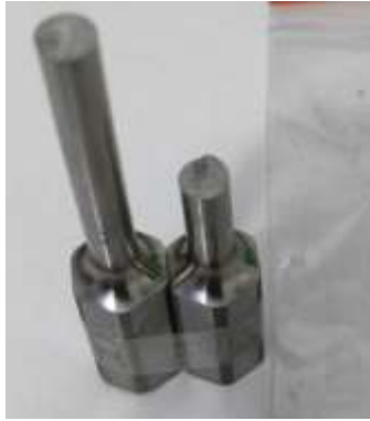
Figure 7. Sample after torsion test
