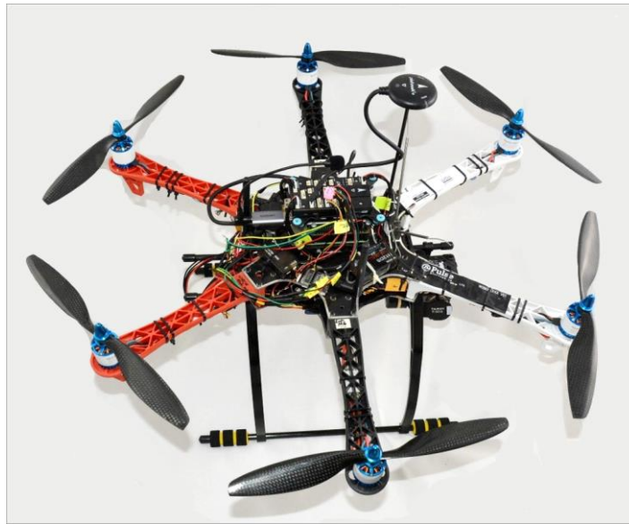
Figure 2.6: Hexacopter and its Six Engines with Propeller
