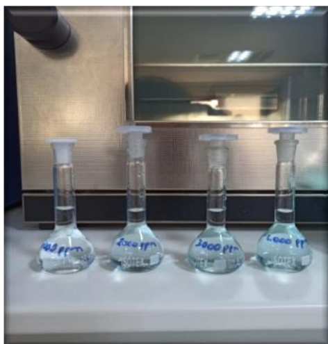
Figure 6. 25 mL 1000, 2000, 3000 and 4000 ppm Cu(II) solution (repeated for each pH value)
