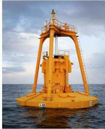
Figure 2. A common example of self-reacting a-body PAs is the OPT Power Buoy gadget [12].
